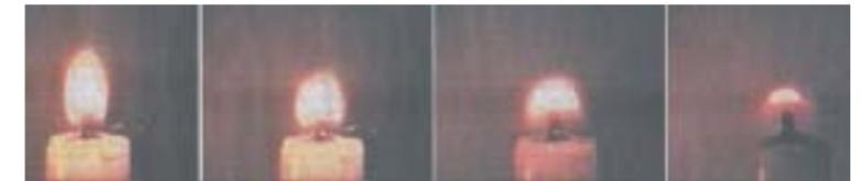
Fig. 1. A candle in the microgravity of a drop tower. The teardrop shape of 1 g (first frame) relaxes towards a sphere.
