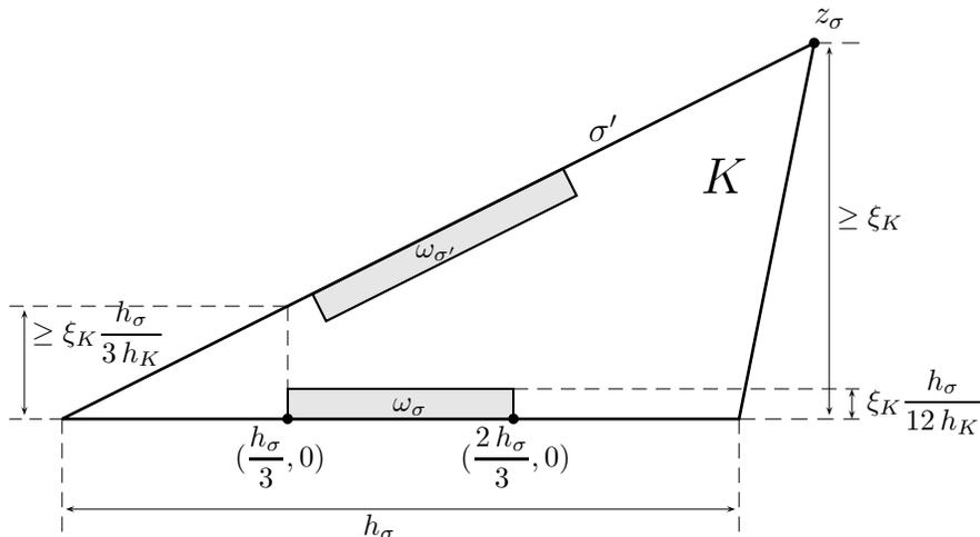
FIGURE 1. Notations for the control volume  $K$
