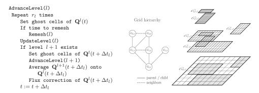
Fig. 2. Recursive AMR algorithm in two dimensions, and typical hierarchy of rectangular submeshes.
