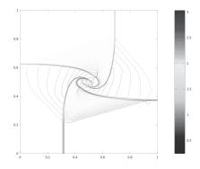
Fig. 3. Left: Reference solution—isolines of density (0  $\leq \rho \leq$  3.2 with step 0.008) at the final time  $t_e$  for the 2D Riemann problem Lax-Liu configuration #6. The computation is performed on a 4096<sup>2</sup> mesh using the FV volume scheme with AUSMDV flux. Right: MR solution, using L=10 and  $\epsilon=0.0023$ .
