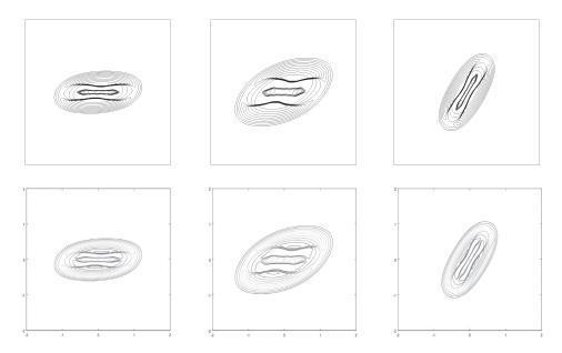
Fig. 5. 3D ellipsoidally expanding shock-wave at time  $t_e$ . Upper row: Isolines of 2D cuts of density for the FV reference solution computed on  $1024^3$  mesh, down-sampled to  $256^3$ , corresponding to L=8. Lower row: Isolines of 2D cuts of density for the MR computation with L=8.
