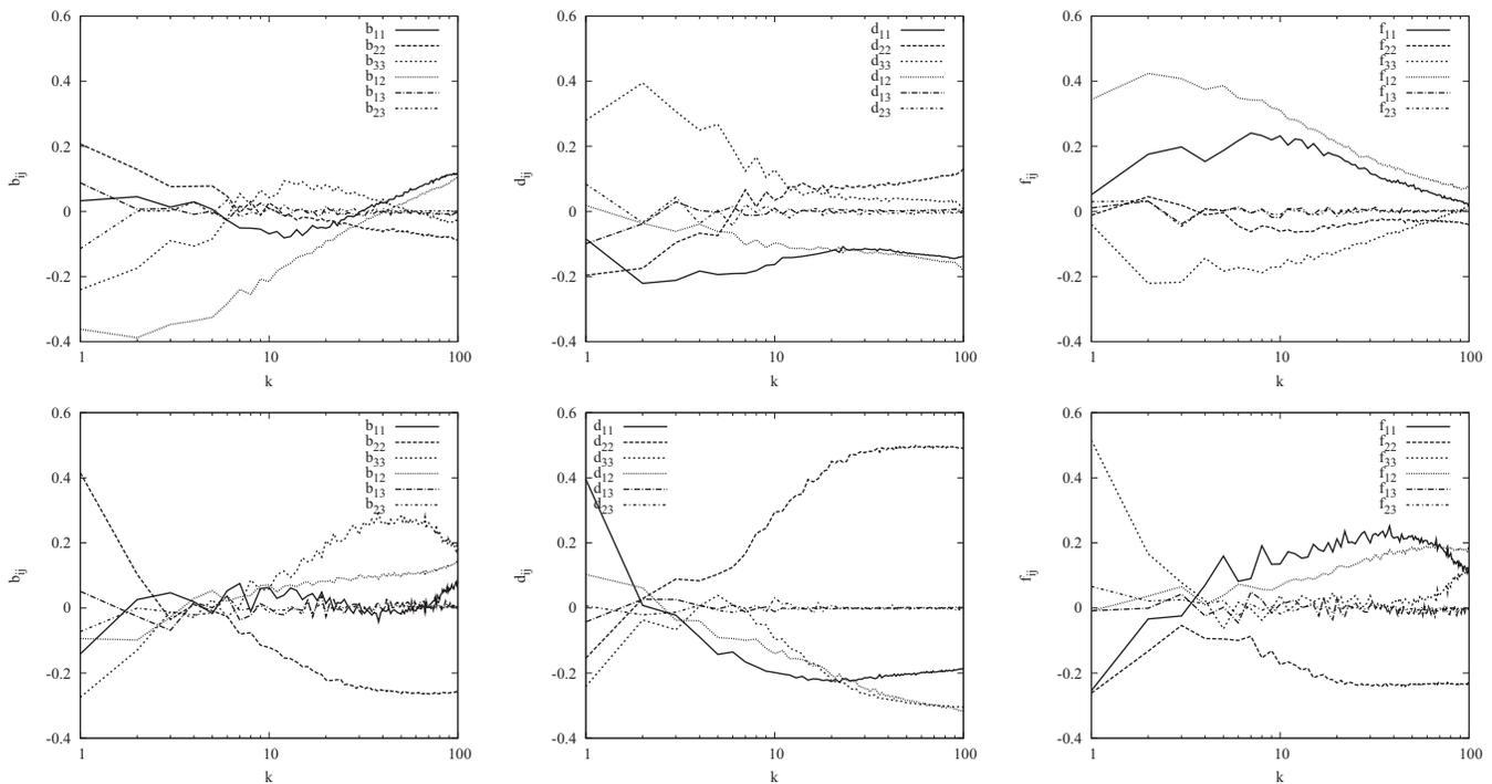
FIG. 8. Wavenumber dependence components of the Reynolds stress anisotropy tensor  $b_{ij}$  (left column), structure dimensionality anisotropy tensor  $d_{ij}$  (center column), and circularity anisotropy tensor  $f_{ij}$  (right column) for two cases with  $f/S=+0.5$  (top row) and  $f/S=+5$  (bottom row) at nondimensional time  $St=5$ .
