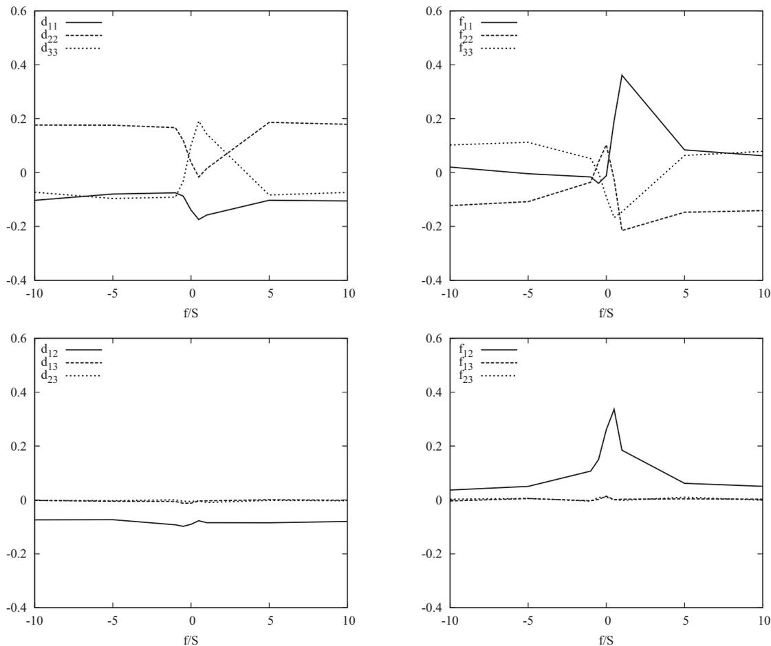
FIG. 7. Dependence of the diagonal components (top row) and off-diagonal components (bottom row) of the structure dimensionality anisotropy tensor  $d_{ij}$  (left column) and the circulatory anisotropy tensor  $f_{ij}$  (right column) on the rotation ratio  $f/S$  at nondimensional time  $St=5$ .
