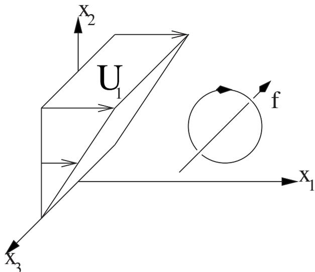
FIG. 1. Schematic of the mean flow configuration with uniform vertical shear  $S = \partial U_1 / \partial x_2$  and rotation  $f = 2 \Omega$ . Note that this schematic shows a parallel configuration with negative rotation ratio  $f/S$ .
