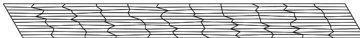
Figure 10. Perturbed parallelogram grid mesh8 with 11 \times 11 cells. To visualize the grid, on this picture the height is 3 times the real height of the grid described in the test case.
