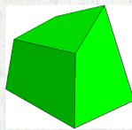
The generalized polyhedral meshes appear in moving mesh (Lagrangian, ALE) methods, in methods fitting a mesh to curved material interfaces, etc.
