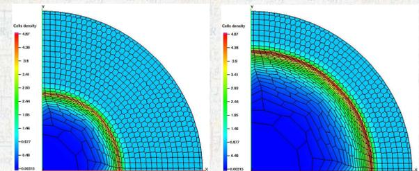
Figure 4: The Sedov explosion problem: a high energy gas is released in a cold gas at point (0, 0). The density profiles at 0.3s and 0.7s illustrate propagation of a shock wave. Lagrangian simulation without artificial viscosity fails at 0.1s.
