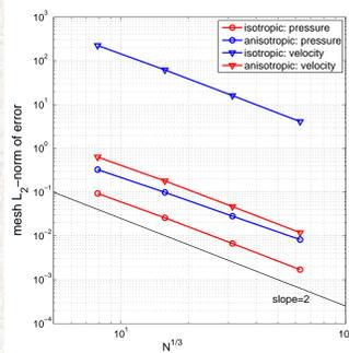
Figure 1: The polyhedral mesh has three spherical layers of prisms. The second-order convergence for  $p^h$  is achieved for both isotropic and anisotropic ( $10^3$ ) diffusion tensors.
