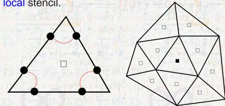
Figure 3: Velocity degrees of freedom are marked by solid circles. Red lines show non-zero off-diagonal entries of matrix  $\mathbb{M}_{\mathcal{F},E}$ . Left picture shows the stencil of  $\mathcal{L}^h$  for the pressure unknown marked by the black square.
