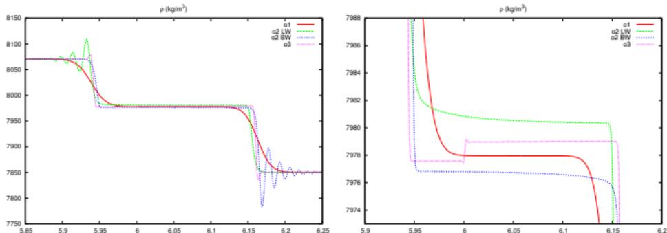
**FIG.:** Right-facing split shock in the Hugoniot experiment on steel for a velocity of 150m/s.
