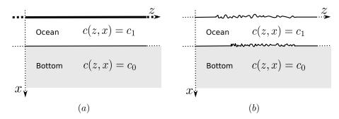
FIGURE 0.1. Illustration of two semi-infinite waveguides with a Pekeris profile. In (a) an unperturbed waveguide with the rigid-lid assumption is considered. In (b) a perturbed waveguide with a free surface and an uneven bottom topography is considered. In the two cases the waveguide are homogeneous in the interior with propagation speed profile c(z,x) equal to  $c_1$  in the ocean section of the waveguide, and  $c_0$  in its bottom.
