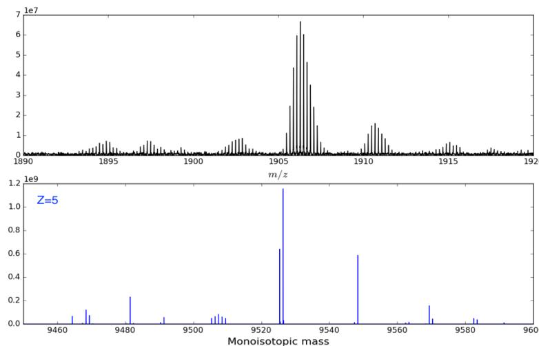
Fig. 2: Analysis of the real FT-ICR-MS spectrum of a peptide in trimer form: (top) zoom on the acquired data; (bottom) recovered spectrum at  $z=5$  using dictionary-based approach.
