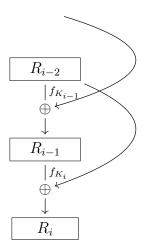
The final output of the Feistel cipher is the inverted pair  $R_rL_r = R_rR_{r-1}$ , which allows the Feistel cipher to be inverted by running through the same algorithm with the key sequence reversed.
