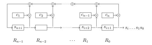
Before discussing the mathematical definition of linear feedback shift registers (LFSR's), we address the question "Why?". A LFSR is essentially an elementary algorithm for generating a keystream, which has the following desirable properties:
