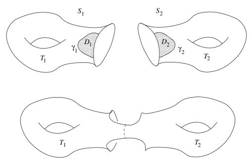
FIGURE 1. The two surfaces  $T_1$  and  $T_2$  are glued together along  $\gamma_1$  and  $\gamma_2$ .
