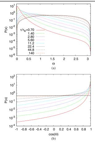
FIG. 3 (color online). PDFs of (a)  $\Theta$  and (b)  $\cos(\Theta)$  for different time lags. Solid black lines indicate the long time asymptotic form of the PDFs.
