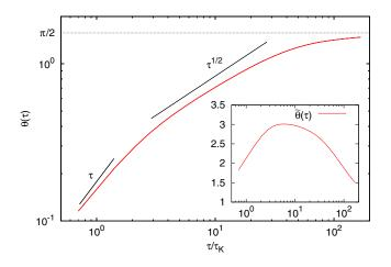
FIG. 2 (color online). The average angle  $\theta$  as a function of the time lag  $\tau$  normalized by the Kolmogorov time scale  $\tau_K$ . In the inset, the compensated angle,  $\tilde{\theta}(\tau) \equiv \theta(\tau) \sigma_u / (\epsilon \tau)^{1/2}$ , is plotted.
