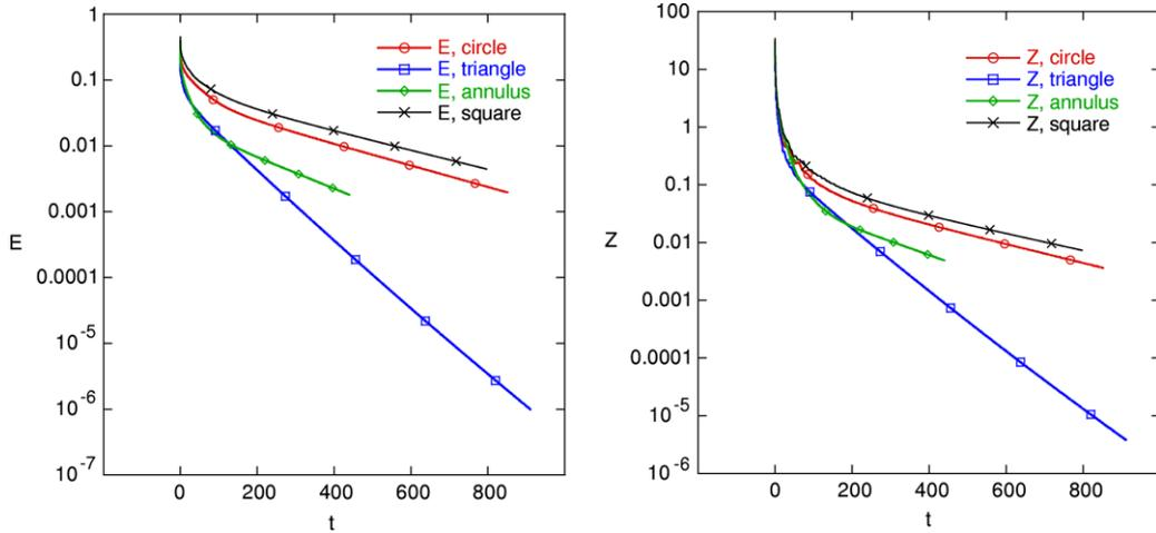
Fig. 2. Decay of energy  $E(t)$  (left) and enstrophy  $Z(t)$  (right) for circular, square, triangular and annular domains.
