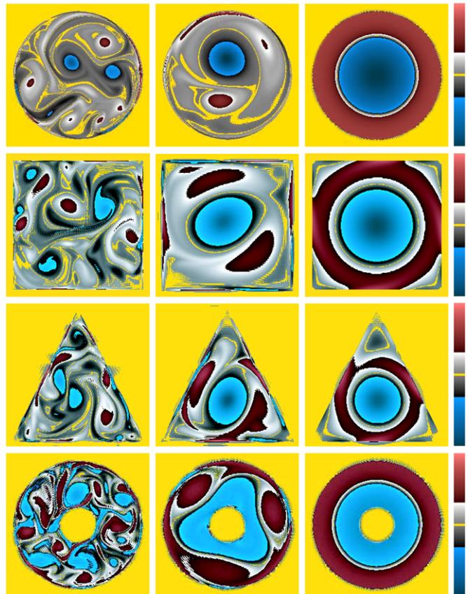
[Fig. 1](#). 2d decaying turbulence in bounded domains. Vorticity fields at early (left), intermediate (middle) and late times (right). From top to bottom: circle, square, triangle and annulus.
