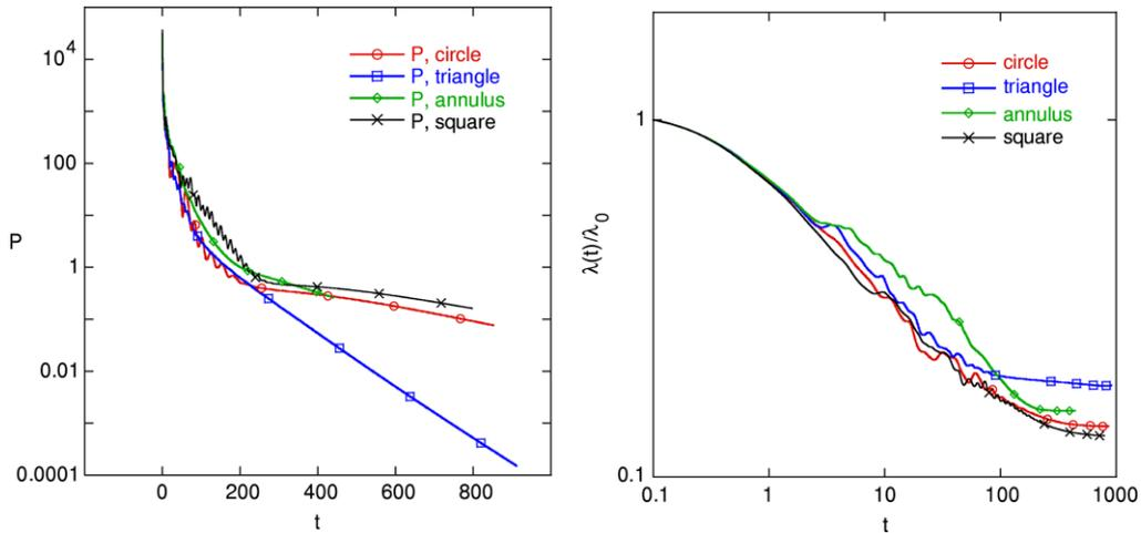
Fig. 3. Decay of palinstrophy  $P(t)$  (left) and the normalized mean square wavenumber  $k_\lambda(t)/k_\lambda(0)$  (right), for circular, square, triangular and annular domains.
