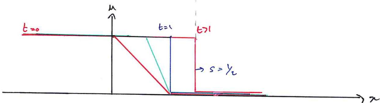
Extending naturally the solution constructed by the method of characteristics beyond  $t=1$ , we look for a weak solution in the domain  $\{t > 1\}$  such that  $u_L(t) = 1$  and  $u_R(t) = 0$ .
