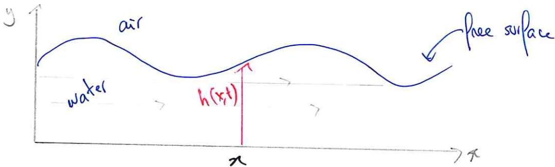
$U(x, y, t)$ : horizontal speed of the incompressible fluid.
