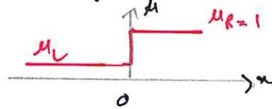
We expect a shock type solution with a discontinuity travelling back to the left. We look for a weak solution of the form:
