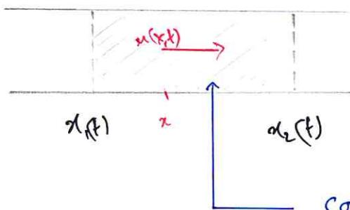
control volume of fixed mass, moving with the flow velocity.
