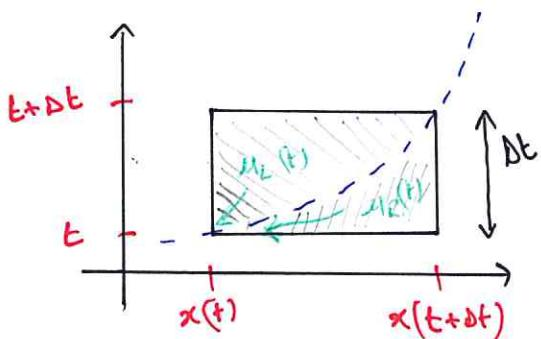
$$\begin{aligned} \alpha(t+dt) &= \alpha(t) + s(t)dt + O(dt^2) \\ \Rightarrow dx &= \alpha(t+dt) - \alpha(t) = s(t)dt + O(dt^2) \\ \Rightarrow \frac{dx}{dt} &= s(t) + O(dt) \end{aligned}$$
