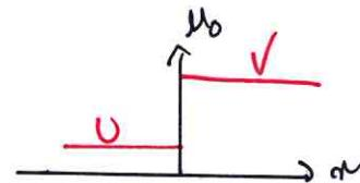
If  $U > V$ , the solution of the Riemann problem is a shock propagating at the speed  $s = \frac{U+V}{2} > 0$  because  $U, V > 0$ .
