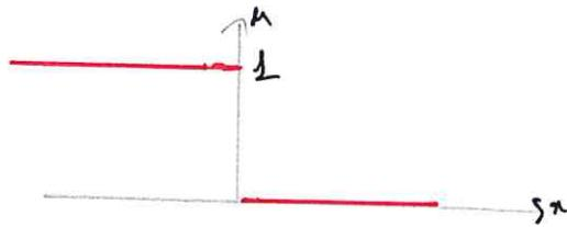
$$\text{Shock speed: (R.H)} \quad \alpha'(t) = \frac{f(u_R) - f(u_L)}{u_R - u_L} = \frac{0}{-1} = 0.$$
