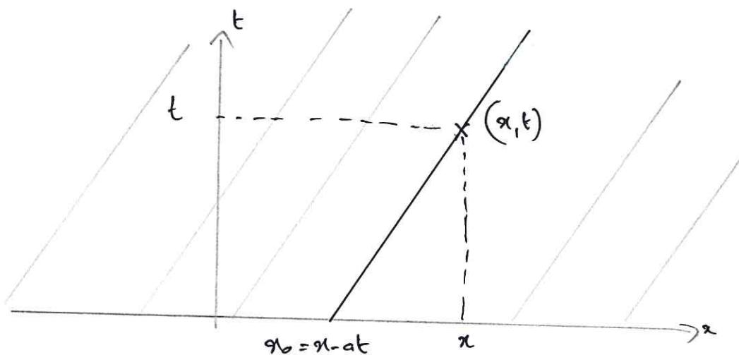
The solution is constant along the characteristics:
