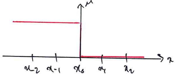
We know that the exact solution is a shock propagating at speed  $s = \frac{1}{2}$ .
