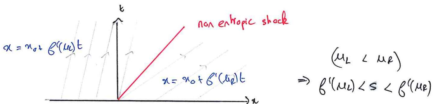
For an entropic shock, the characteristics must enter into the shock.
