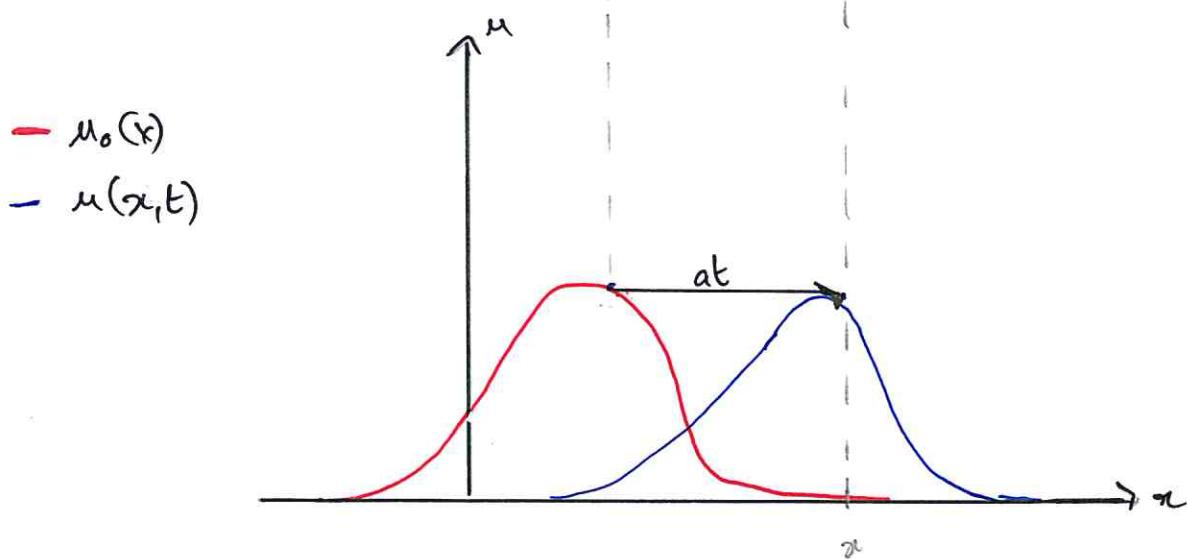
The initial condition  $u_0$  is simply transported at the speed  $a$ .
