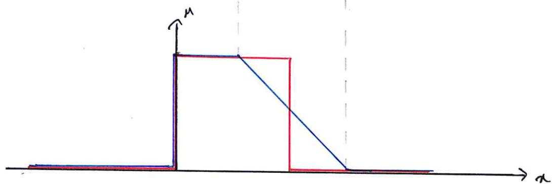
Shock speed  $= 0 >$  Speed of the left boundary of the rarefaction wave  $= -\frac{1}{2}$ .
