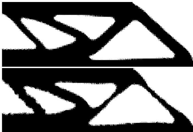
Figure 24: BBM beam initial (top) and final (bottom) shapes for the test case of Section 5.3.2.
