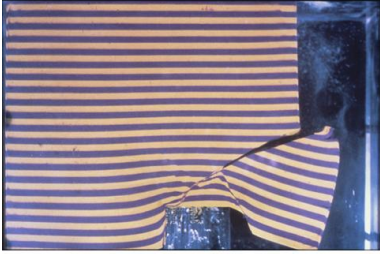
Figure 19: Tapponnier and Peltzer's indentation experiment.
