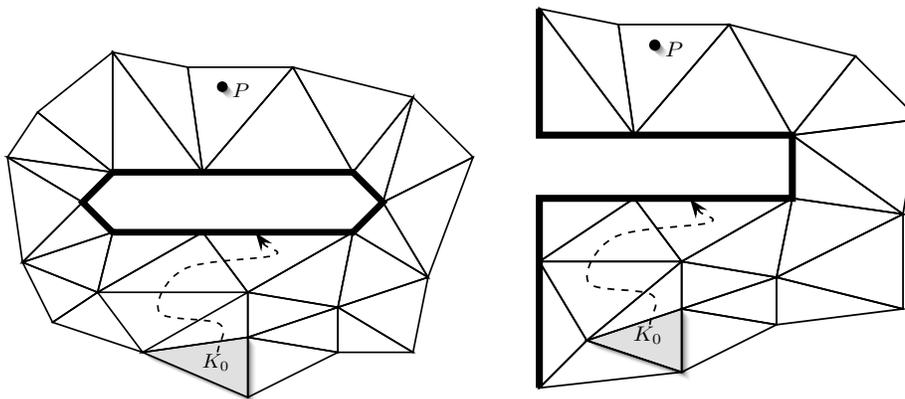
Figure 4. *Starting element  $K_0$  and vertex  $P$  are separated by a hole (left) or the non-convex domain (right). The path demands to pass through the hole or the boundary to reach the element containing vertex  $P$ .*
