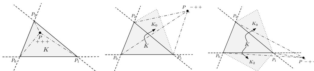
Figure 2. Illustration of the three possible cases depending on the signs of the three barycentric coordinates of vertex  $P$  with respect to triangle  $K$  when moving inside the background mesh.
