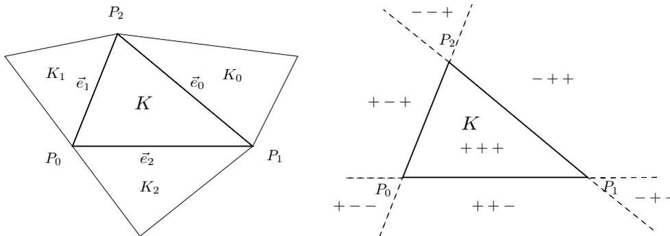
Figure 1. Left, definition of a triangle  $K$  and its three neighbors  $K_i$ . Vertices indices are ordered counter-clockwise and the entities numeration is the same as the viewing vertices. Right, the seven regions defined by the signs of the three barycentric coordinates of a point  $P$  with respect to an element  $K$ .
