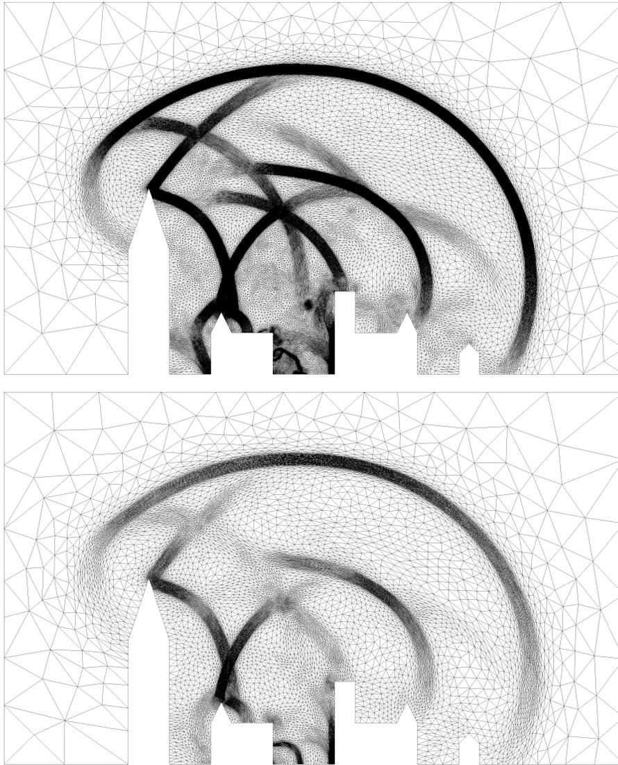
Figure 23. Final adapted meshes using the  $\mathbf{P}^1$ -conservative interpolation at time  $t = 0.2$  seconds for errors equal to 0.003 (top) and 0.006 (bottom). The upper mesh contains 170,020 vertices and the lower one 23,767.
