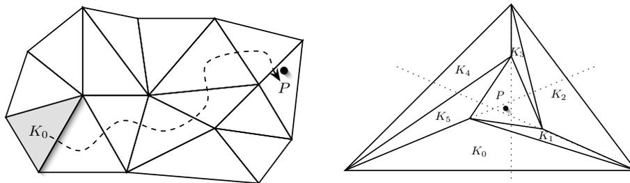
Figure 3. *Left, a possible path to locate the vertex  $P$  of the new mesh starting from the triangle  $K_0$  of the background mesh. Right, cyclic path leading us to an already checked element. Starting from  $K_0$ , triangles  $K_1$ ,  $K_2$ ,  $K_3$ ,  $K_4$  and  $K_5$  are visited bringing us back to  $K_0$ .*
