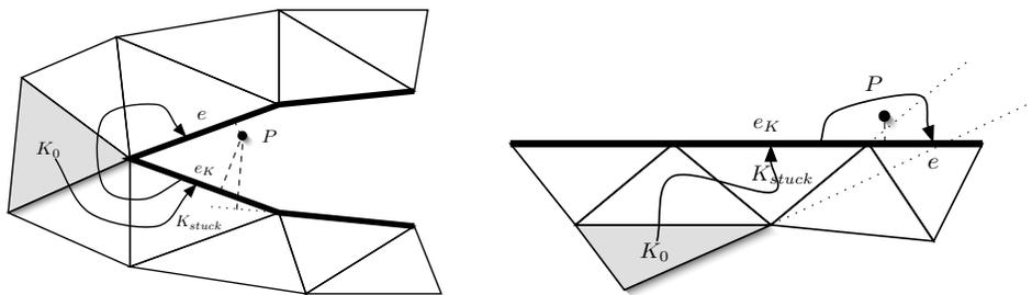
Figure 7. Illustration of the possible cases when a vertex is outside of the domain. The localization algorithm ends in triangle  $K_{stuck}$ . The condition (i) (resp. (ii)) is not fulfilled for edge  $e_K$  on the left (resp. right) figure. We have to move to edge  $e$  to find the "closest" triangle.
