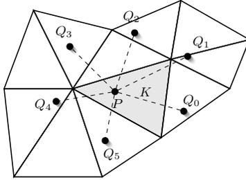
Figure 5. Reducing the number of visited triangles in the localization scheme by using the topology of both meshes. Vertex  $P$  has been located in element  $K$ . Then, the set of vertices  $\{Q_i\}_{i=1,m}$  connected to  $P$  uses element  $K$  as initial guess for the localization scheme.
