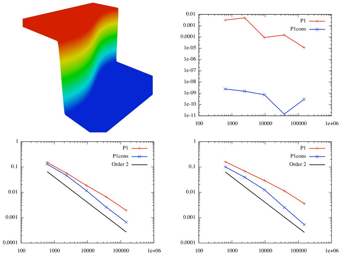
Figure 13. Continuous sinusoidal shock analytical function  $f_2$ . Top left, a three-dimensionnal representation of the function. Top right, the mass variation for the transfer  $\mathcal{H}_i^1 \rightarrow \mathcal{H}_i^2$ . Bottom left, the error  $\epsilon_i$  for the transfer  $\mathcal{H}_i^1 \rightarrow \mathcal{H}_i^2$ . Bottom right, the error  $\epsilon_i$  for the transfer  $\mathcal{H}_i^1 \rightarrow \mathcal{H}_i^2 \rightarrow \mathcal{H}_i^1$ .
