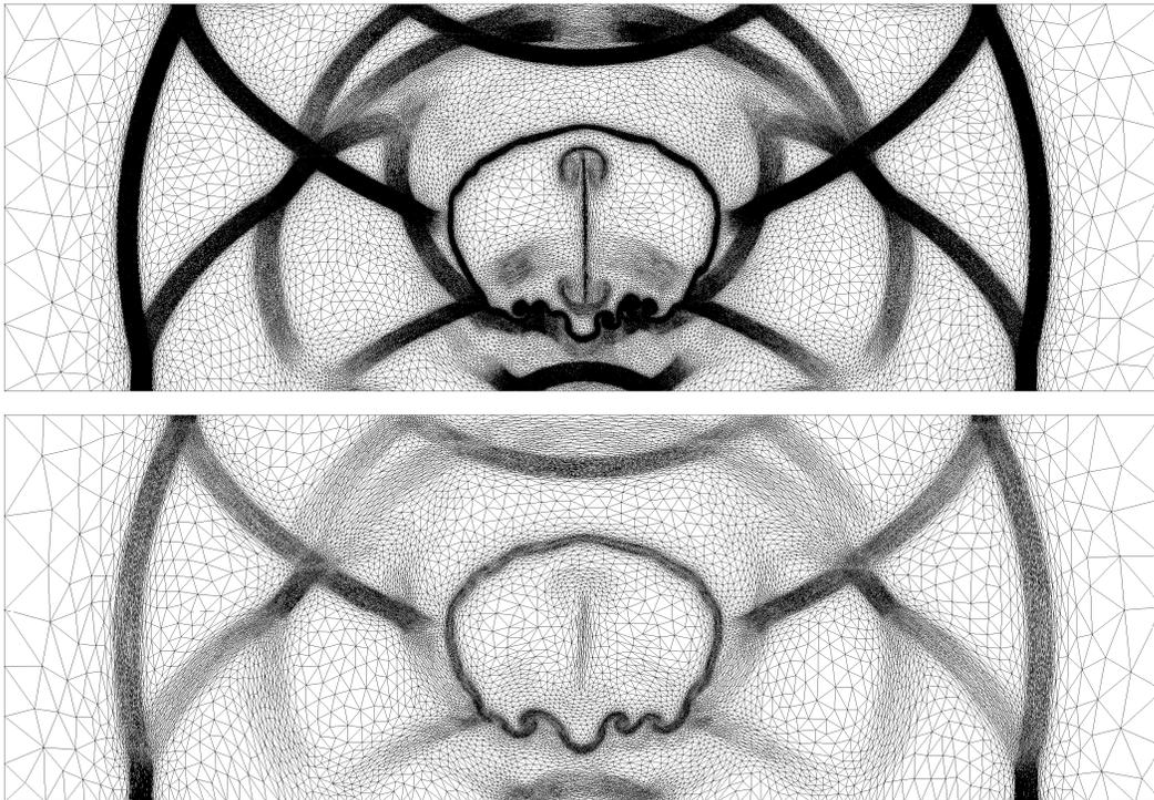
Figure 18. Final adapted meshes using the  $P^1$ -conservative interpolation at time  $t = 0.7$  for errors equal to 0.015 (top) and 0.03 (bottom). The upper mesh contains 158,121 vertices and the lower one 24,297.
