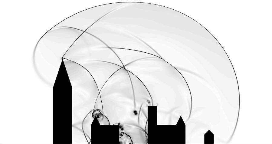
Figure 21. A schlieren type picture representing the final density at  $t = 0.2$  sec on the final adapted mesh containing 170,020 vertices obtained from an error level of 0.003 and the  $\mathbf{P}^1$ -conservative interpolation.
