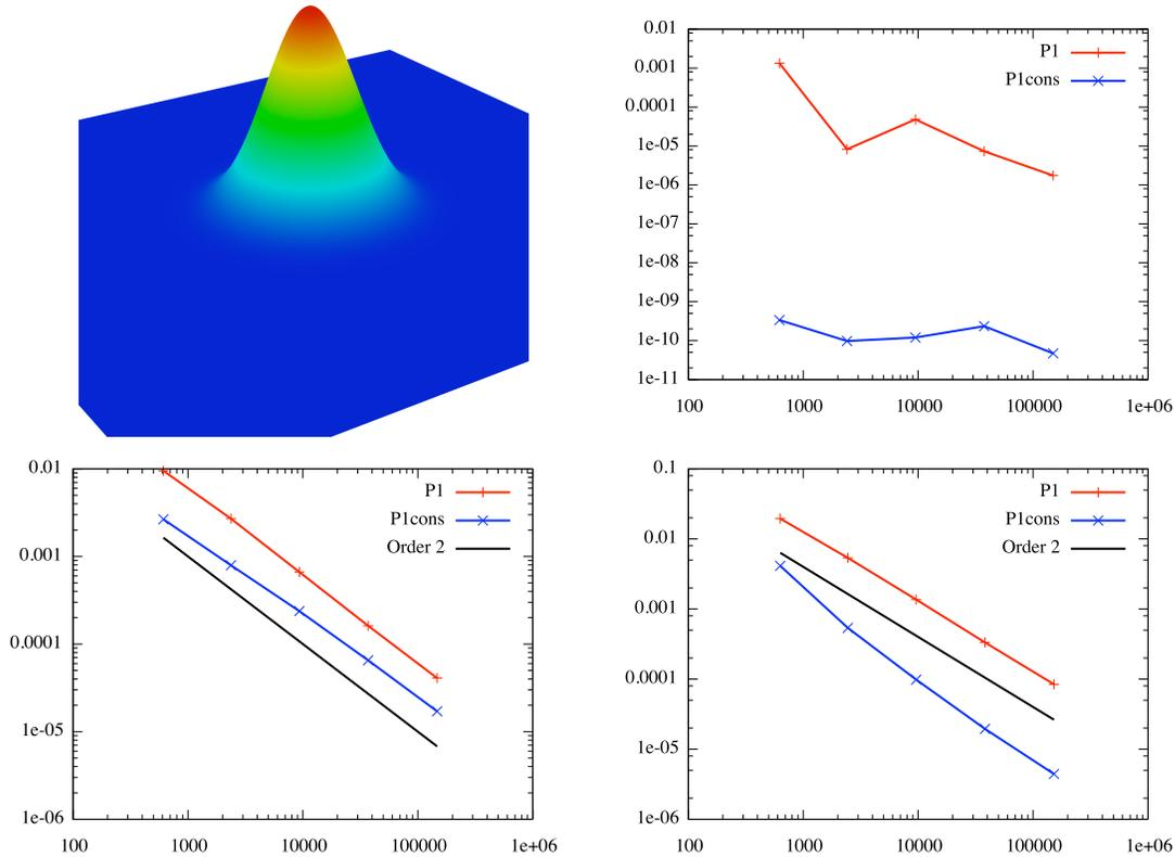
Figure 12. Gaussian analytical function  $f_1$ . Top left, a three-dimensionnal representation of the function. Top right, the mass variation for the transfer  $\mathcal{H}_i^1 \rightarrow \mathcal{H}_i^2$ . Bottom left, the error  $\varepsilon_i$  for the transfer  $\mathcal{H}_i^1 \rightarrow \mathcal{H}_i^2$ . Bottom right, the error  $\epsilon_i$  for the transfer  $\mathcal{H}_i^1 \rightarrow \mathcal{H}_i^2 \rightarrow \mathcal{H}_i^1$ .
