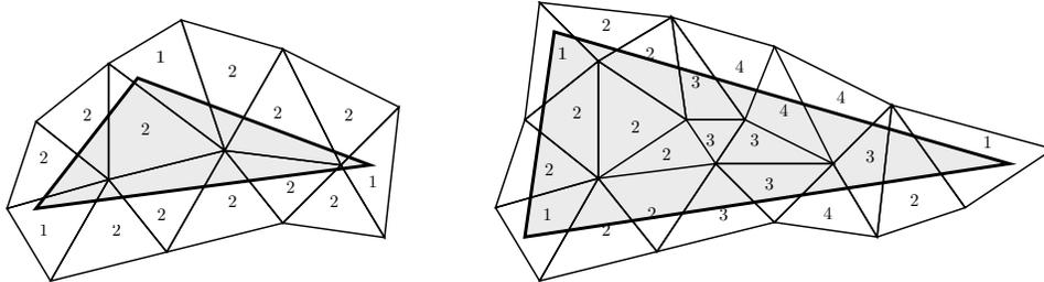
Figure 10. *Illustration of the overlapped elements detection process. First, the list of the background elements to which the vertices of  $K^{new}$  belong are detected: they are tagged 1. Then, the other elements are iteratively detected while computing intersections. The tag number represents the intersection step. Two steps are sufficient for the left case, whereas the right case requires four steps.*
