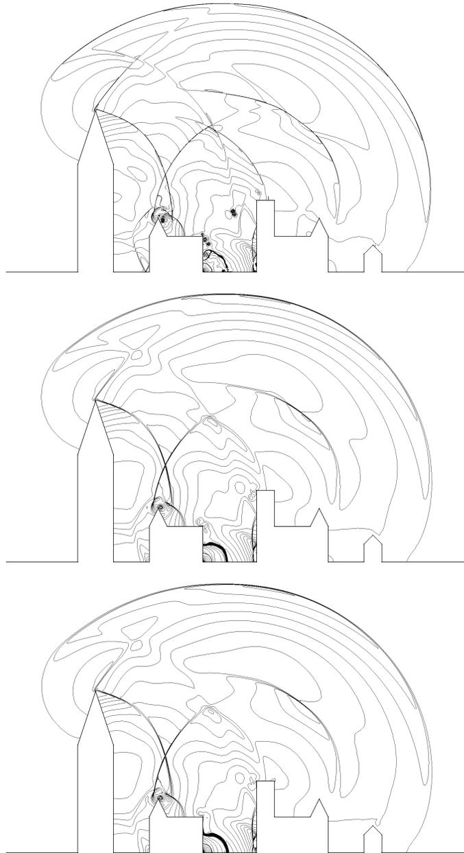
Figure 24. Density isolines from 0.085 to 0.19 with an increment of  $2.65 e^{-3}$  at time  $t = 0.2$  seconds. Top, the reference solution, i.e.,  $\varepsilon = 0.003$  and the  $P^1$ -conservative interpolation. Middle, adapted solution obtained for  $\varepsilon = 0.006$  with the  $P^1$ -conservative interpolation. Bottom, adapted solution obtained for  $\varepsilon = 0.006$  with the  $P^1$ -interpolation.
