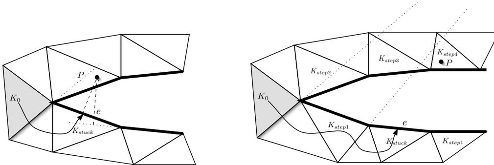
Figure 6. Two illustrations of the "fork" problem when the algorithm has made the wrong choice. We are stuck in triangle  $K_{stuck}$  where  $P$  is viewed by boundary edge  $e$ . The figure on the right illustrates the process to remedy this problem by restarting the localization from new triangles. At first step, we choose triangles  $K_{step1}$  as initial guess. Then,  $K_{step2}$  if  $P$  has not been found. And so on.
