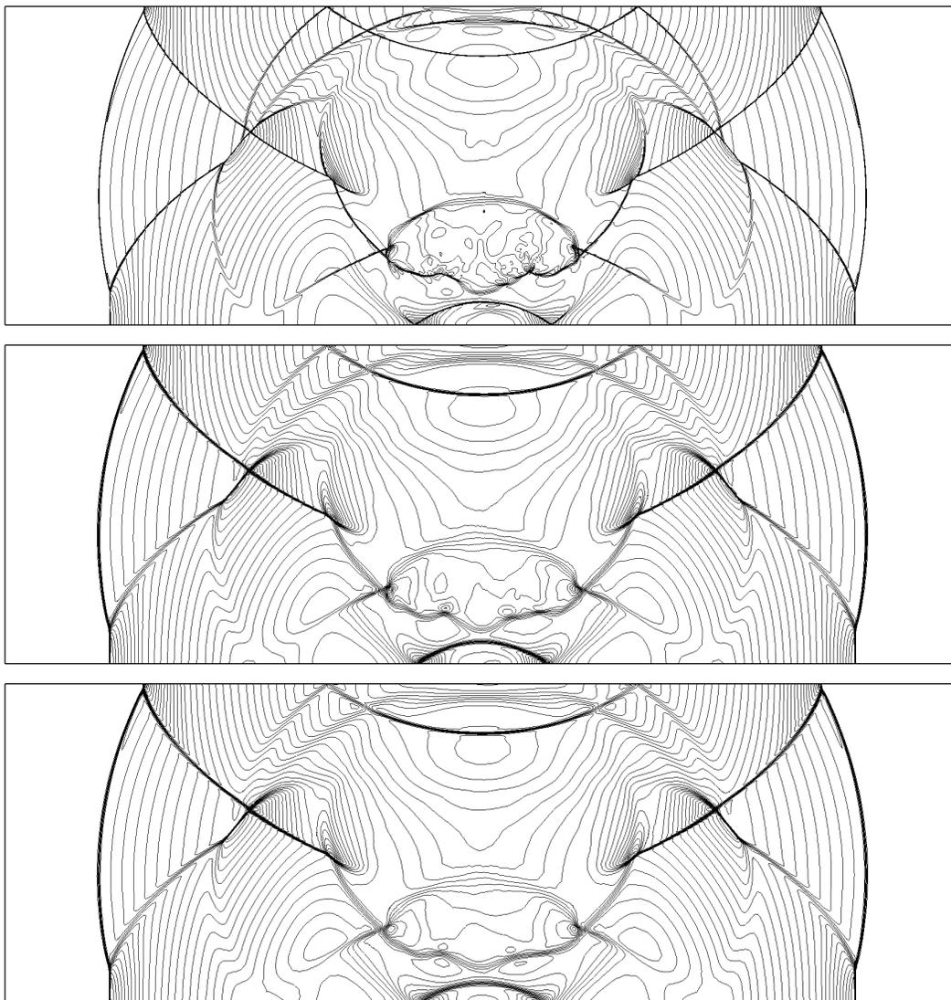
Figure 19. Pressure isolines from 0.715 to 1.695 with an increment of 0.0245 at time  $t = 0.7$ . Top, the reference solution, i.e.,  $\varepsilon = 0.015$  and the  $\mathbf{P}^1$ -conservative interpolation. Middle, adapted solution obtained for  $\varepsilon = 0.03$  with the  $\mathbf{P}^1$ -conservative interpolation. Bottom, adapted solution obtained for  $\varepsilon = 0.03$  with the  $\mathbf{P}^1$ -interpolation.
