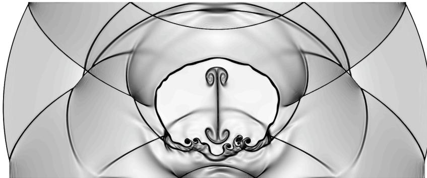
Figure 17. A schlieren type picture representing the final density at  $t = 0.7$  on the final adapted mesh containing 158,121 vertices obtained from an error level of 0.015 and the  $\mathbf{P}^1$ -conservative interpolation.
