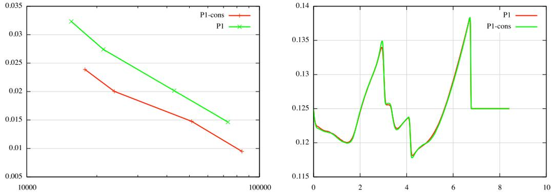
Figure 25. Left,  $L^2$ -norm error of the density with respect to the reference solution for adaptive simulations for  $\varepsilon$  from 0.007 to 0.004. In red, adaptive simulations with the  $\mathbf{P}^1$ -conservative interpolation and, in green, with the  $\mathbf{P}^1$  interpolation. Right, comparison of the density profile at time  $t = 0.2$  seconds along the line of equation  $y = 3.07692x - 17.4615$  for the solutions obtained with an error threshold  $\varepsilon = 0.006$ .
