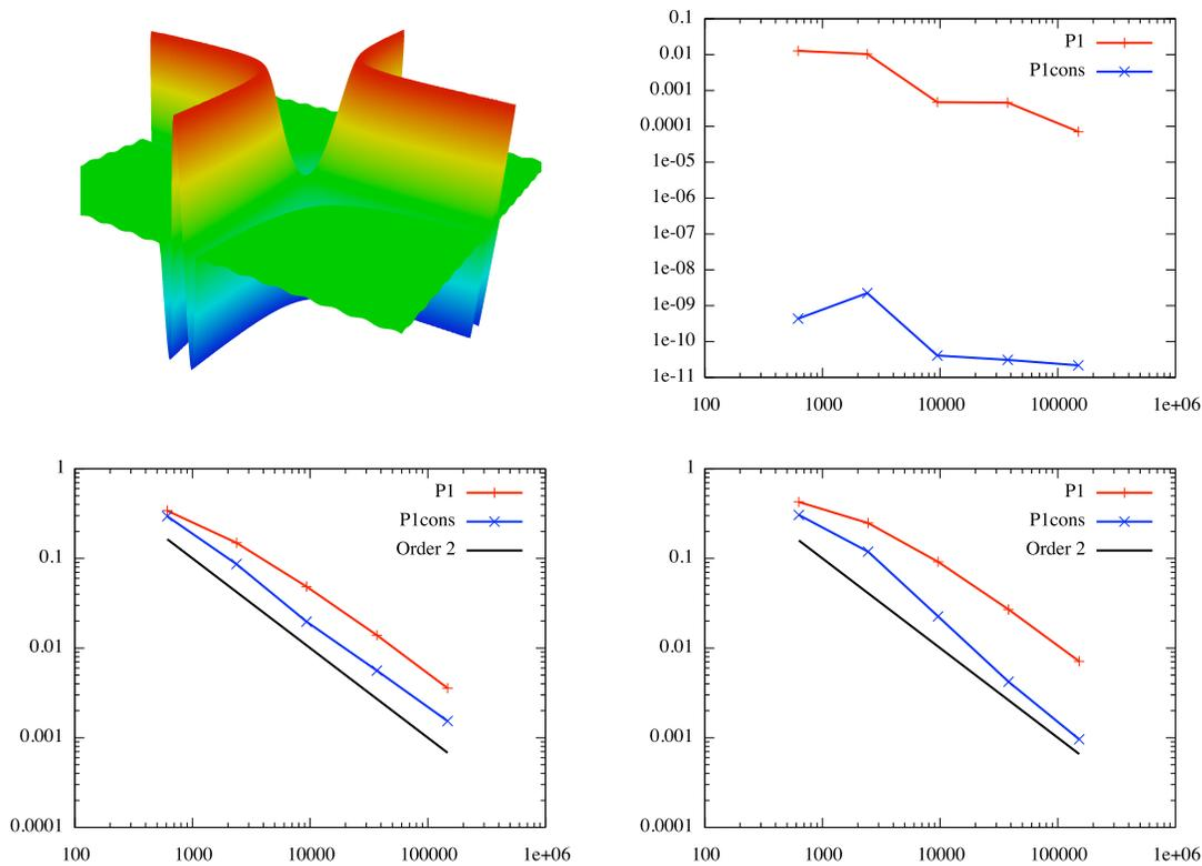
Figure 14. Multi-scales smooth analytical function  $f_3$ . Top left, a three-dimensionnal representation of the function. Top right, the mass variation for the transfer  $\mathcal{H}_i^1 \rightarrow \mathcal{H}_i^2$ . Bottom left, the error  $\epsilon_i$  for the transfer  $\mathcal{H}_i^1 \rightarrow \mathcal{H}_i^2$ . Bottom right, the error  $\epsilon_i$  for the transfer  $\mathcal{H}_i^1 \rightarrow \mathcal{H}_i^2 \rightarrow \mathcal{H}_i^1$ .
