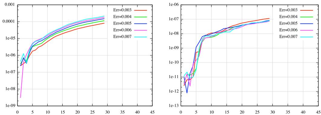
Figure 26. Density relative mass variation during the simulation for all cases. The abscissae represent the iterations of the mesh adaptation algorithm. Left, mass variation for the  $\mathbf{P}^1$  interpolation. Right, mass variation for the  $\mathbf{P}^1$ -conservative interpolation.
