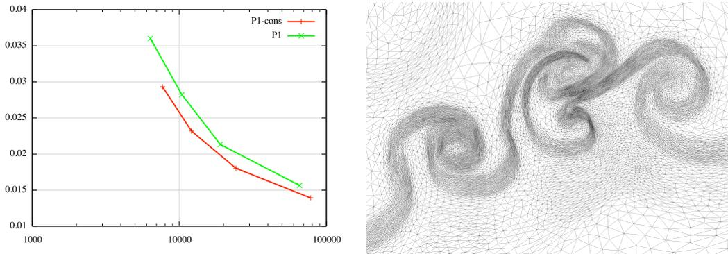
Figure 20. *Left,  $L^2$ -norm error of the density with respect to the reference solution for adaptive simulations for  $\varepsilon$  from 0.05 to 0.02. In red, adaptive simulations with the  $\mathbf{P}^1$ -conservative interpolation and, in green, with the  $\mathbf{P}^1$  interpolation. Right, a close up view of the adapted mesh of Figure 18 (top) in a region where instabilities occur.*
