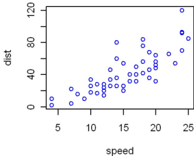
Figure: Distance de freinage
