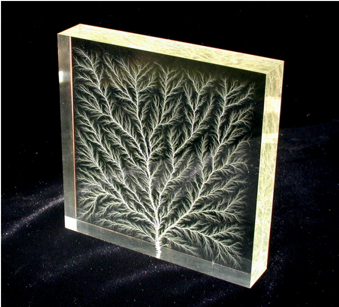
DLA in art: "High-voltage dielectric breakdown within a block of plexiglas" (from Wikipedia)
