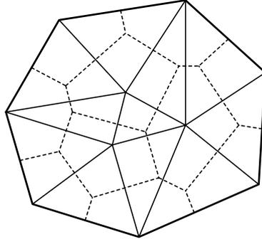
FIGURE 1. Continuous line: Finite Element mesh. Dashed line: Voronoï mesh associated to the vertices of the Finite Element mesh.
